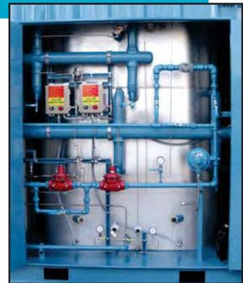
Pneumatic Process Control Standard, Electro-Mechanical Control Available
